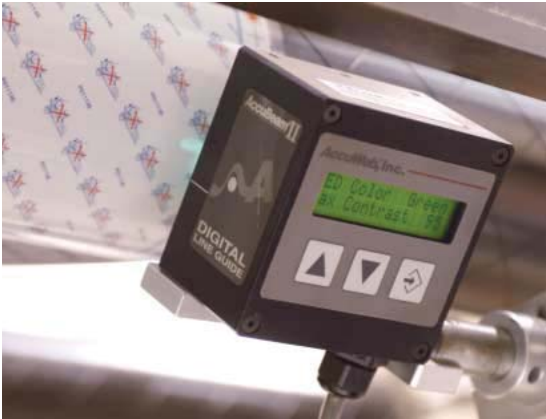
AccuBeam® II digital line guides on Alcan's Kampf slitler/rewinders (left) provide optimum contrast on reflective foil laminates. AccuWeb HT-4 explosion-proof electromechanical linear actuators (below) were retrofitted in all of Alcan Packaging Pharma's Class I Div. I environments.
